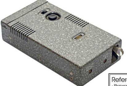
Left hand side and front view of the Czech elbug keyer. The paddle was on the right hand side of the front along with pre-set controls of mark and space. The variable speed could be adjusted with a thumb wheel control on top of the unit. A mains fuse and on-off switch were located at the top rear.
